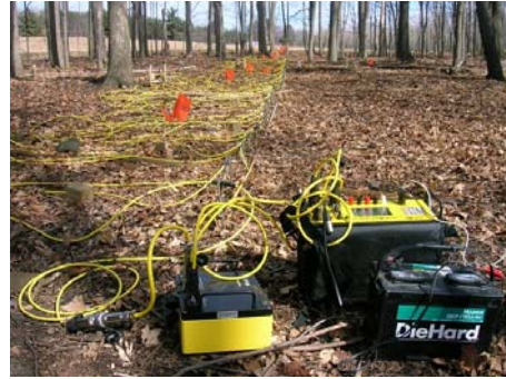
AGI SuperSting R8 IP Earth Resistivity and IP Meter assembly.
